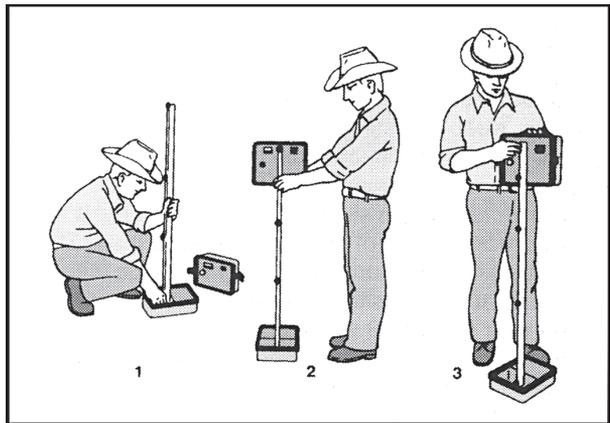
**Figure 5.** Assembly for Narrow Scan Inductive Search
