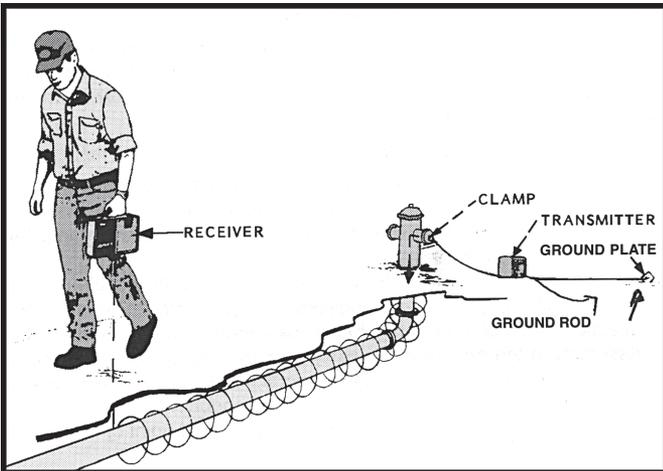
Figure 9. Conductive Trace
